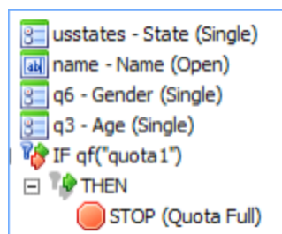
Figure 32 Stop node to disposition interviews when a quota cell is filled
