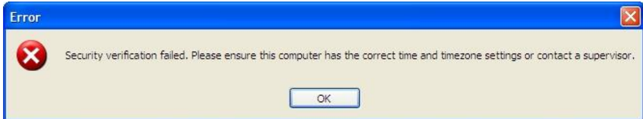
Figure 238 Warning message displayed if the interviewer computer system time does not correspond to the UTC
